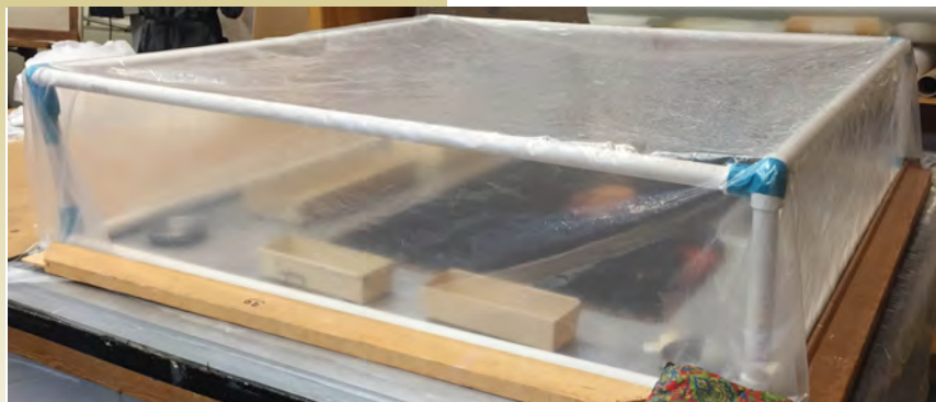
Top: Alexa Beller inpainting losses near the completion of treatment. Inset: Alexa mending a tear and securing a canvas insert into a loss in the canvas. Above: The painting before treatment in specular light highlights the slackness of the original canvas; the painting was placed in a humidity chamber. (Images: Albertson, Schneck, Beller.)
