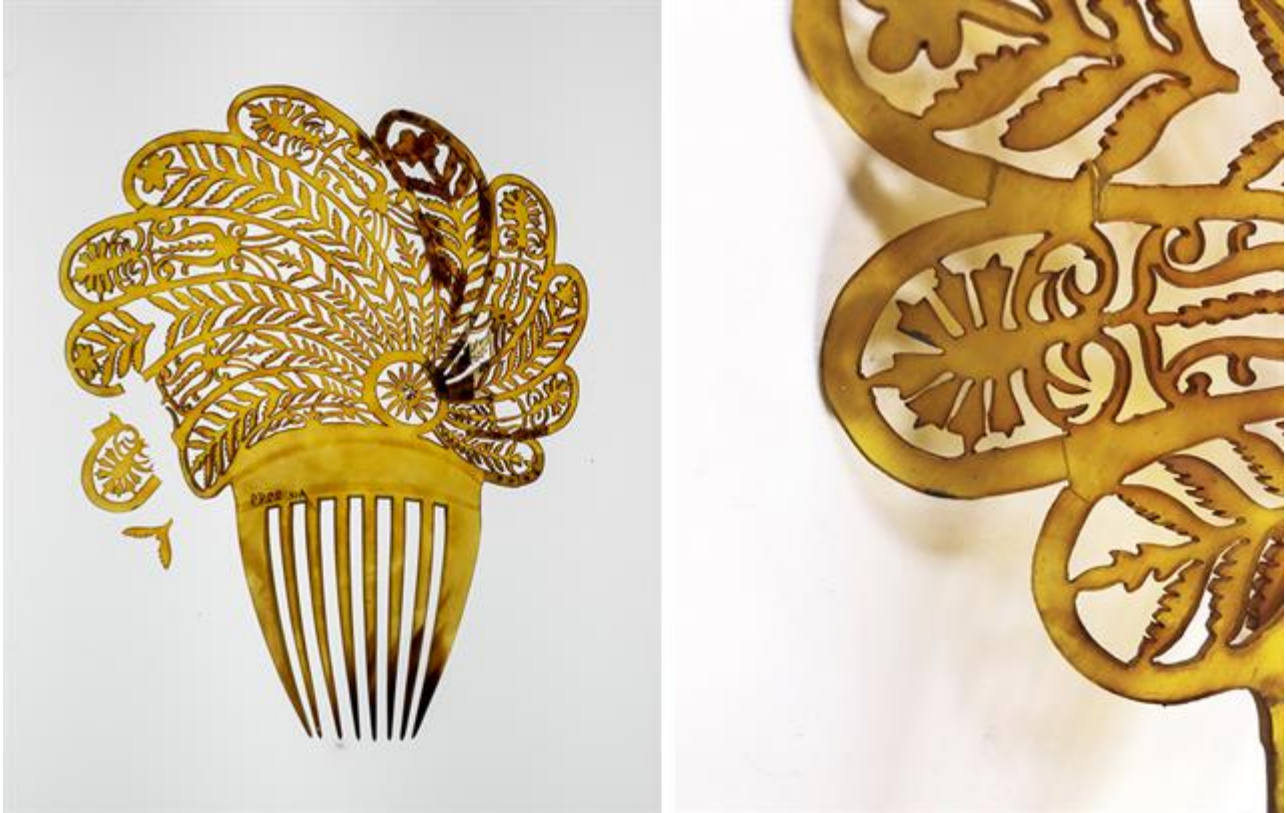
Early plastics include cellulose nitrate, which was used in the production of this hair comb. (Images courtesy of Abigail Rodriguez.)
