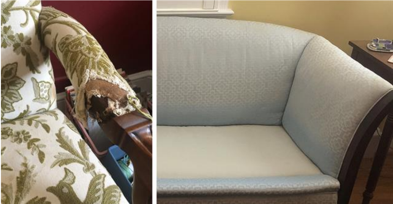
Left: The result of an over-eager dog anxiously awaiting the return of his owner and using the arm of this chair as a chew toy. (Image courtesy of Allison Kelley.) Right: This couch has experienced a heavy dose of light damage. The original color is still present where the seat cushion protected some of the upholstery. (Image courtesy of Amanda Kelley.)
