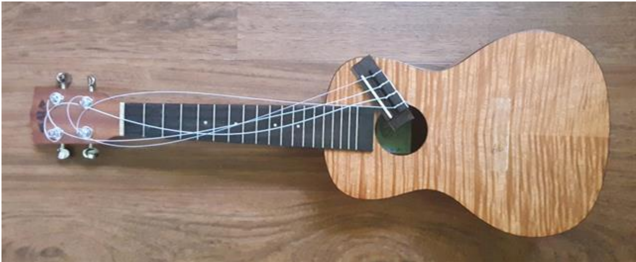
A 20th-century ukulele. The saddle and bridge, which had been glued to the wooden body under tight tension from its four nylon strings, had become detached during a move. The instrument experienced a rapid change in temperature and humidity in its environment, which caused the wood body and nylon strings to expand and contract so extremely that the glued bridge popped off. Fortunately, this damage was treatable and the ukulele could be repaired. (Image courtesy of Emily Brzezinski.)
